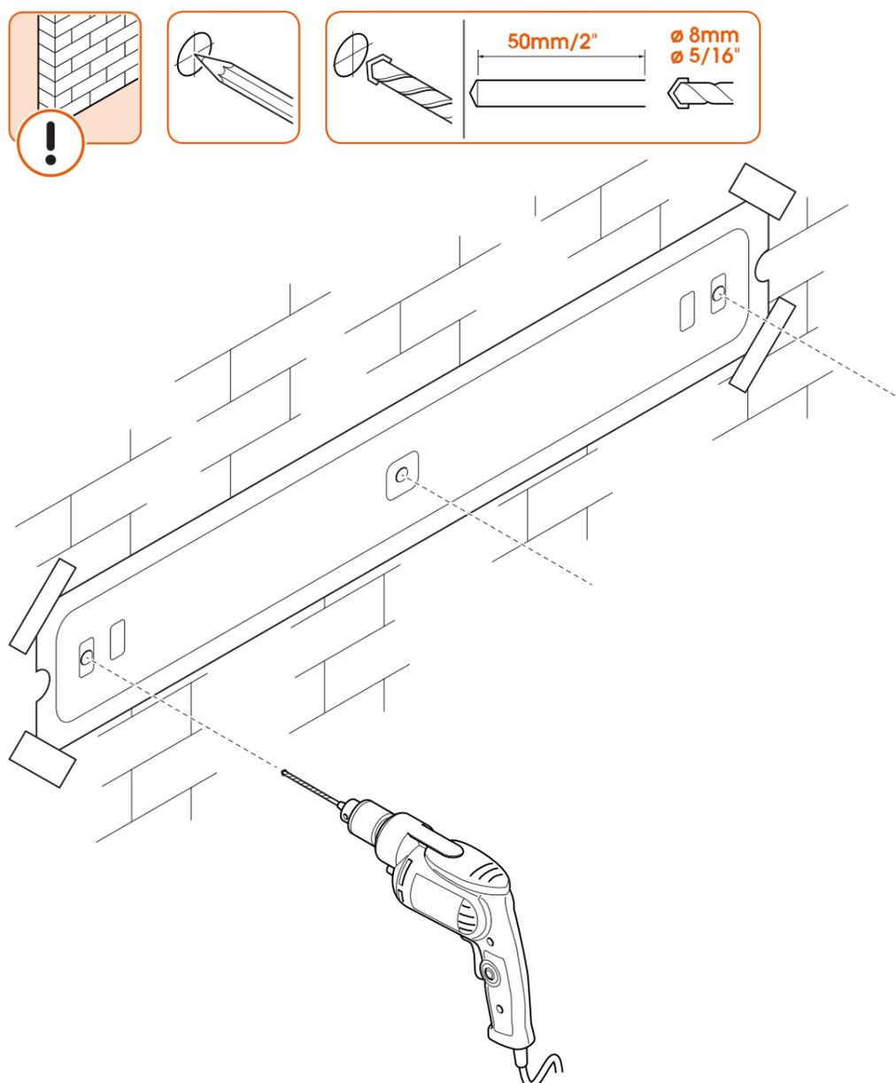
1. Find the perfect spot for drilling with our [DrillRight™ AR app](#) and the included drilling template.
