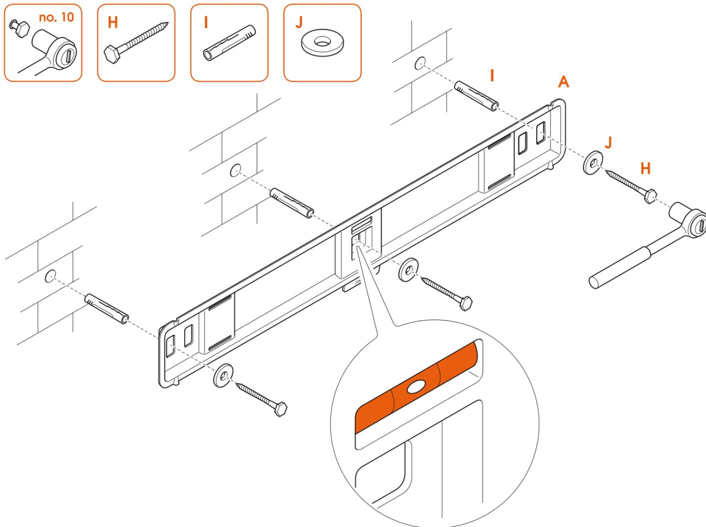
3. Attach the **wall mount** (A) to the wall with the **screws** (H), **washers** (J) and **plugs** (I). Use the spirit level to level the wall mount.
