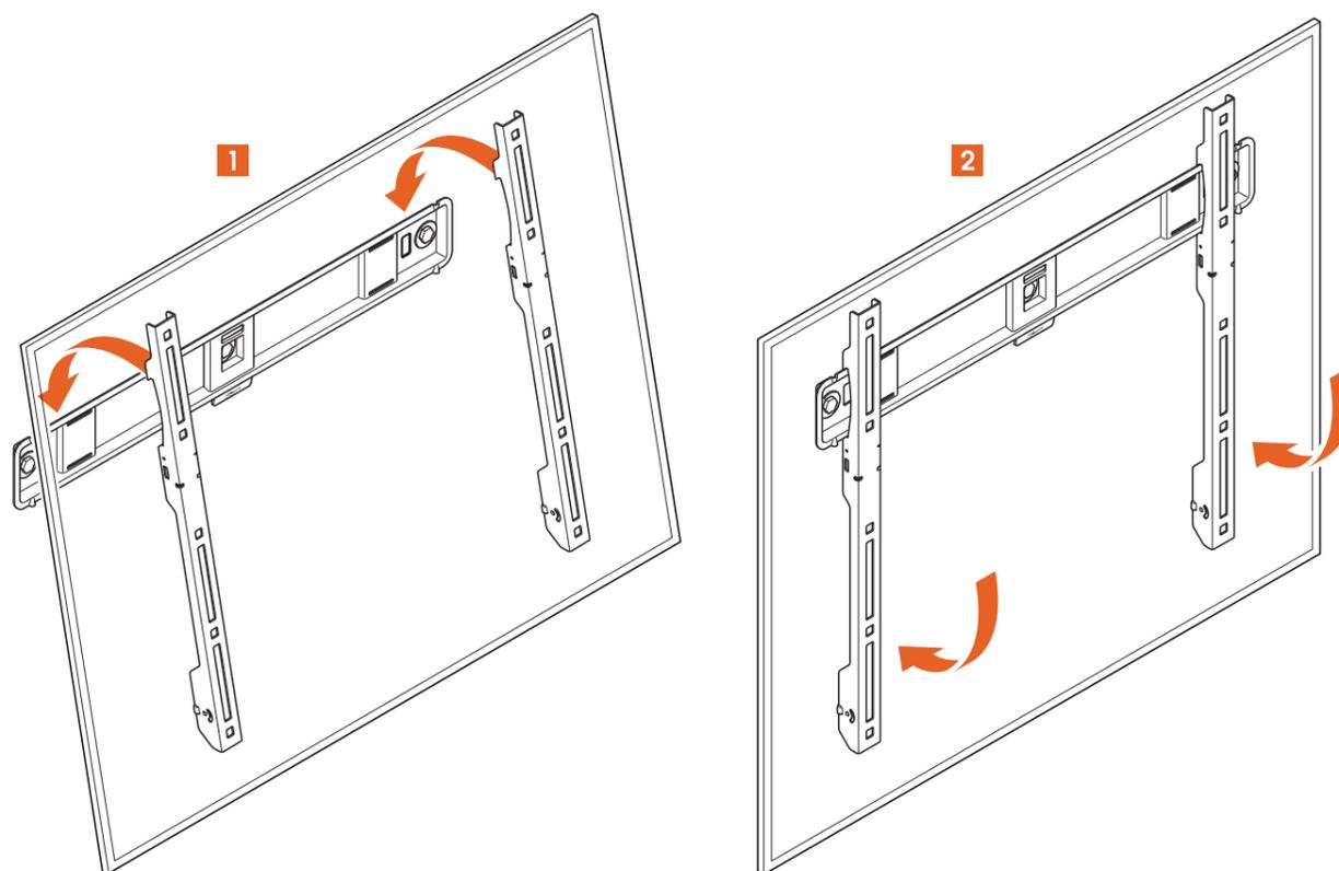
1. Carefully lift and attach the TV to the wall mount (A).
