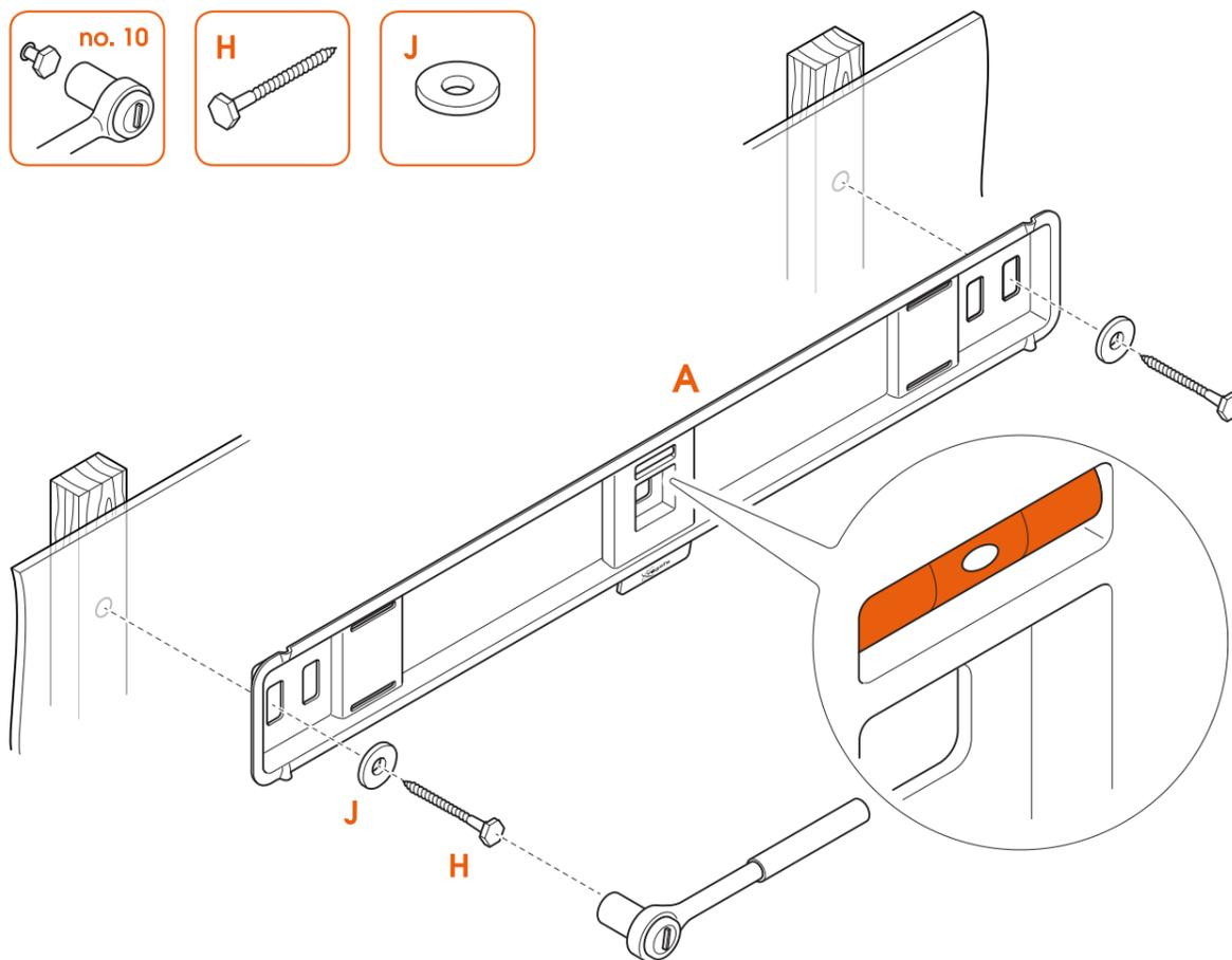
4. Attach the **wall mount** (A) to the wooden wall with the **screws** (H) and **washers** (J). Use the spirit level to level the wall mount.
