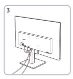
Put both cables in the cable holder on the stand (HOLDER-STAND CABLE) to organise the cables, as shown in the figure.
