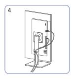
Put both cables in the cable holder on the stand (HOLDER-STAND CABLE) to organise the cables, as shown in the figure.
